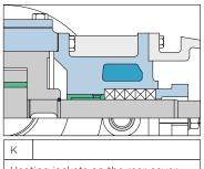
Heating jackets on the rear cover, often required prior to start-up when pumping high-viscosity liquids and liquids which tend to solidify. This jacket is also used as a seal cooling jacket.
