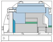
Heating jackets on the front cover, often required prior to start-up when pumping high-viscosity liquids and liquids which tend to solidify.
