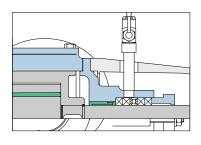
Sealing with stuffing box, with or without lantern ring, for use of external lubrication. Used for high viscosities and where some leakage is allowed.
