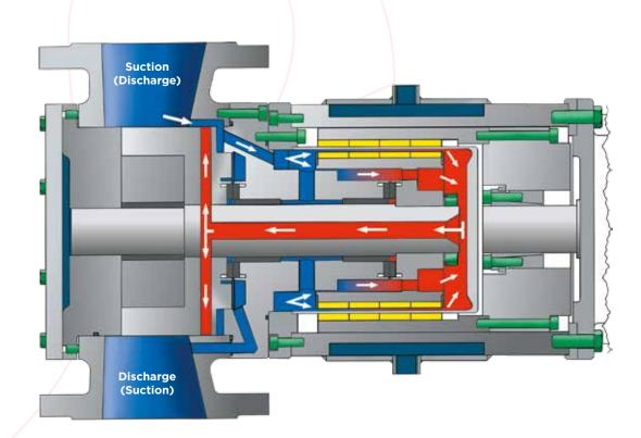
One of the distinguished features of the ROTAN<sup>®</sup> ED range is that the pumped medium is hermetically contained in the system since the magnetic coupling eliminates the need for a shaft and mechanical seal, which could allow gaseous exchange between the pumped medium and the atmosphere.
