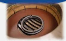
Seal faces are lapped to within one or two light bands. We offer a state-of-the-art facility with specialists dedicated to seal repairs. Every seal must pass a 40 psi pressure test before leaving our facility.
